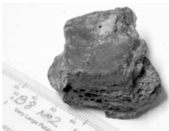
**Illus 6** Cindery sample of partially melted very fine-grained sandstone or mudstone. Note the abundance of cavities formed by expanding gas and that they form trains following the original bedding. From grid square B8. Stone is 5cm across.
